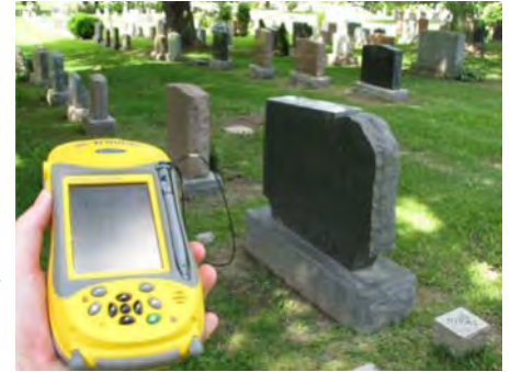
GIS professionals can use your existing maps, CAD drawings, and aerial imagery or go on-site with a high-resolution GPS data logger to locate your plots, roads, buildings, iconography, signage, gardens, trails, trees, niches, crypts and memorials. (LEES+Associates)
